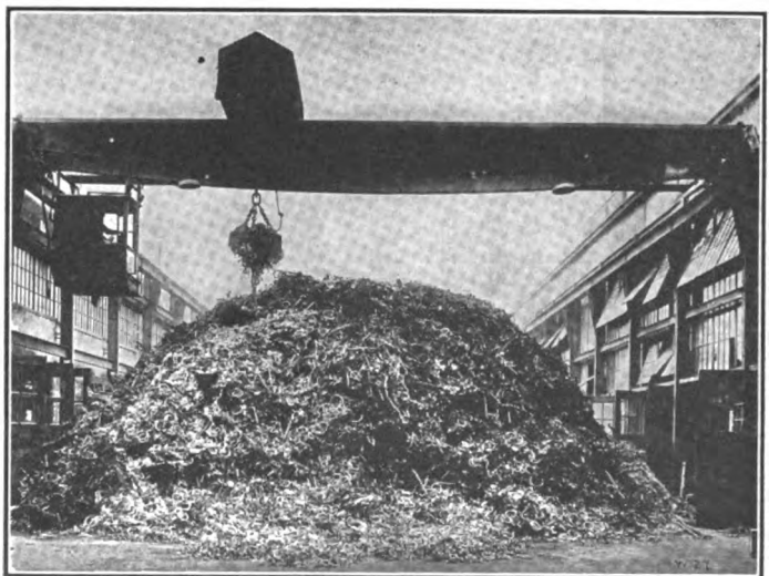
Electro-magnet dumping scrap in Detroit
